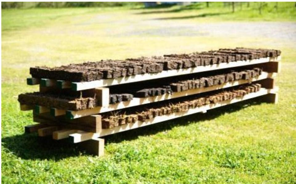
*Briquettes drying in the sun – a 2-3 day process in warm, dry weather*
