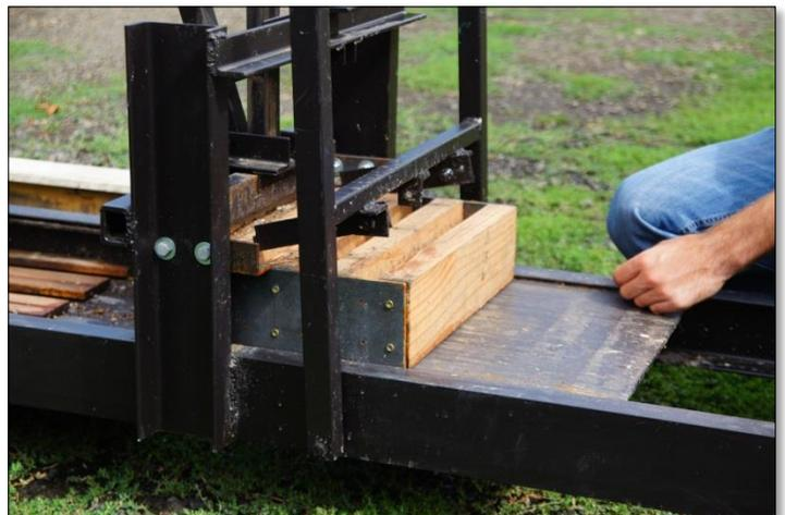
*Detail of the press magazine used to form briquettes*
