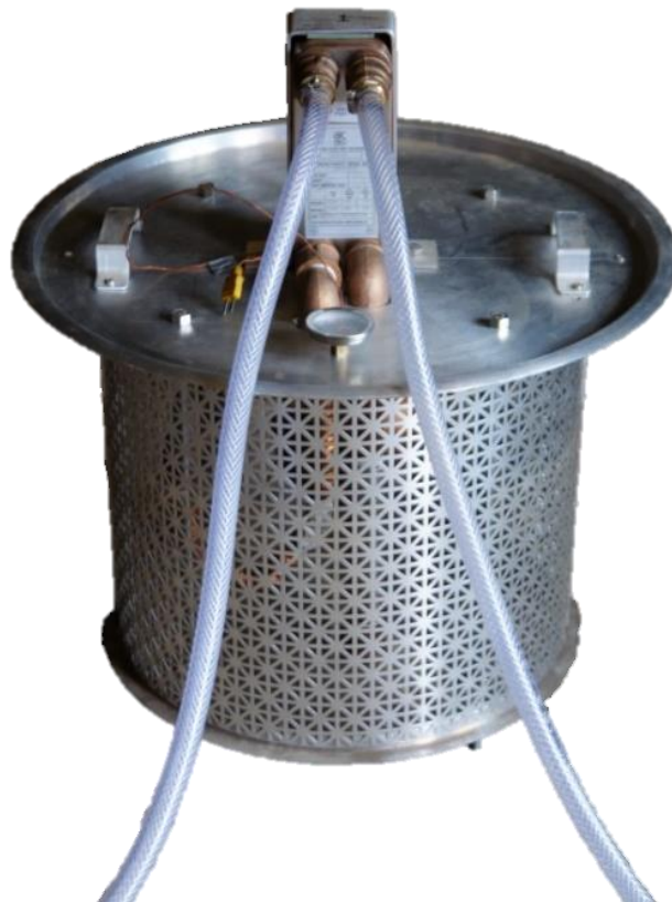
Pasteurizer is mounted on a modified 100L pot lid
