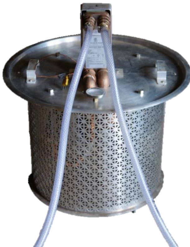
Pasteurizer is mounted on a modified 100L pot lid
